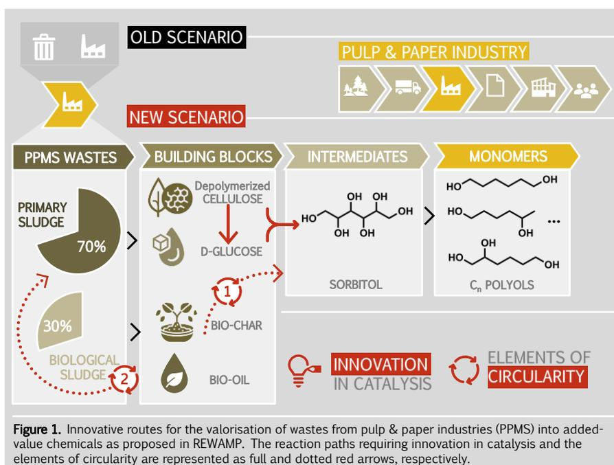
**Figure 1.** Innovative routes for the valorisation of wastes from pulp & paper industries (PPMS) into added-value chemicals as proposed in REWAMP. The reaction paths requiring innovation in catalysis and the elements of circularity are represented as full and dotted red arrows, respectively.
